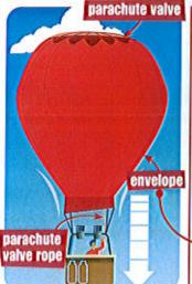
Step 2: To move the balloon down, the pilot pulls the parachute valve rope. It pulls down the parachute valve and hot air goes out of the envelope. When there is less hot air in the envelope, the balloon goes down.
