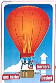
Step 1: To move the balloon up, the pilot releases gas. The burner heats it. Hot air rises and so the hot air lifts the basket off the ground. The more gas that is released, the higher the balloon goes.
