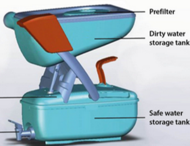
Safe water tap
